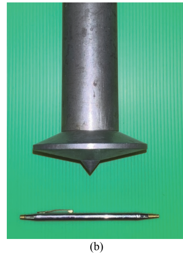
Fig. 5 Shape and dimensions of model spudcan
