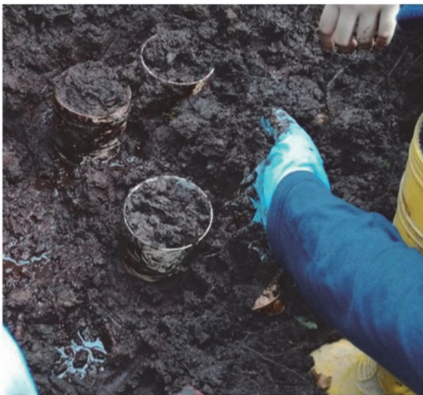
Fig. 2 Picture showing the undisturbed sampling method
